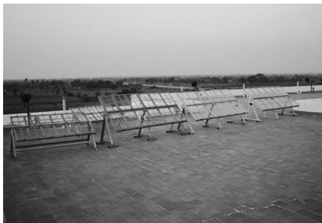
Figure 1 Outdoor exposure racks used for natural weathering studies.
